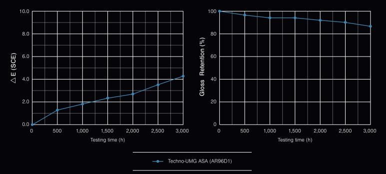
Accelerating Weathering Test (ASTM G155 Cycle1)
