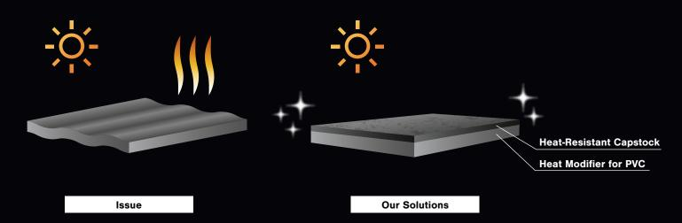
Dark colored profiles absorb heat resulting in visual and quality problems such as warping (left). Techno-UMG is your one-stop shop that offers heat protection in two ways:
